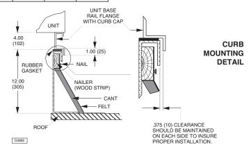
Roof Curb kits ship dis-assembled for ease of handling and storage. All kits ship complete with mounting hardware (for unit to curb), insulation, gasketing, sealant and installation instructions for field mounting.
